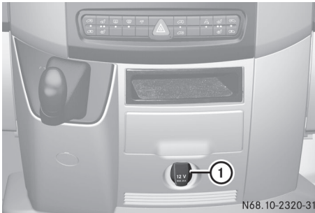
Socket on the lower section of the center console ① 12 V socket, 25 A
