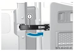
• Vehicles with 270° pivoting rear doors: If you prefer to keep door retainer • out of the loading area when loading the vehicle, you can swivel it 180° against the spring force and onto the door and engage it. The door retainer remains in this position and will not swivel back to its original position.
