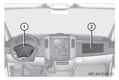
Driver's front air bag (1) deploys in front of the steering wheel; co-driver's front air bag (2) deploys in front of and above the glove box. They are deployed:
