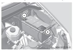
Additional battery in the engine compartment
