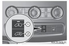
If the automatic locking when driving function is activated, there is a risk of being locked out when the vehicle is pushed or towed.
