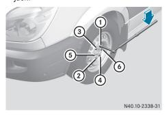
Tightening torque pattern
