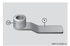
Valve tool with handle and turning piece
