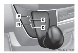
When the selector lever is in position **D**, the automatic transmission selects the individual gears automatically. This depends on:
