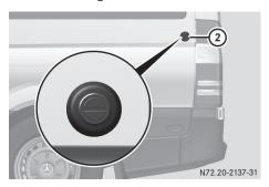
▶ With the rear door opened to an angle of 270°, push it against magnetic door retainer (2) on the side wall. When the magnet on the rear door is in contact with magnetic door retainer (2), the rear door is held in this position.
