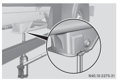
Jacking point (example: Cab Chassis)
