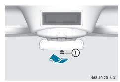
► Anti-glare mode: push anti-glare lever ① in the direction of the arrow.
