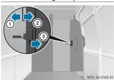
▶ To unlock: press the catch in the direction of arrow (3).
