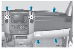
Air vents (example: right-hand side of the vehicle) You can use the air vents to ventilate the
