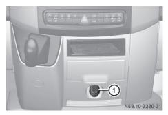
Socket on the lower section of the center console (1) 12 V socket (25 A)
