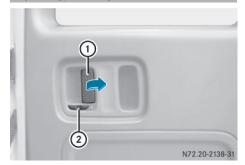
Release the lever on the inside of the right rear door.
