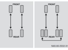
Diagram showing tire rotation for single and dual tires
