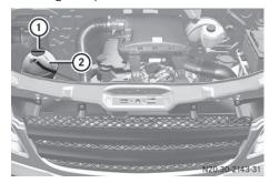
Example: cap and coolant expansion tank
