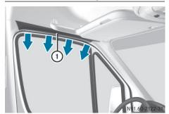
Window curtain air bags ① enhance protection for the head (but not the chest or arms) of the vehicle occupants on the side of the vehicle on which the impact occurs.
