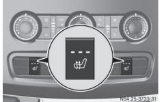
The three red indicator lamps in the #/ button show the activated heating level 1 to 3.
