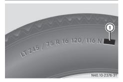
In addition to the load-bearing index, load rating ① may be imprinted after the letters that identify speed rating on the sidewall of the tire ( $\triangleright$  page 302).
