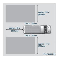
Blind Spot Assist monitors the area approximately 10 ft (3.0 m) behind your vehicle and approximately 11.5 ft (3.5 m) to each side of it. For this purpose, Blind Spot Assist uses radar sensors in the rear bumper and behind the protective strips of the B-pillars.
