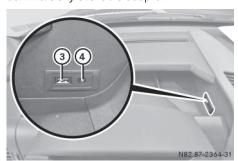
PND connector (on the side behind the instrument cluster)
