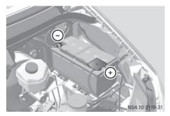
Additional battery in the engine compartment
