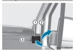
Side air vent (example: right-hand side of the vehicle)
