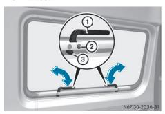
The emergency exit window is intended for use in an emergency only and must not be opened unless the vehicle is stationary. The emergency exit window is the first window behind the driver's seat on the driver's side. It is marked by the "Emergency Exit" label.
