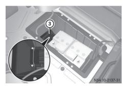
► Loosen the bolts holding retainer ③, which prevents the battery from moving around.
