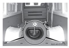
Cargo tie-down point (example: Cargo Van without loading rails)
