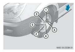
Tightening torque pattern
