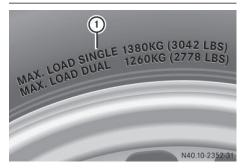
Maximum tire load ① is the maximum permissible weight for which the tire is approved. Do not overload the tires by exceeding the specified load limit. The maximum permissible load can be found on the vehicle's Tire and
