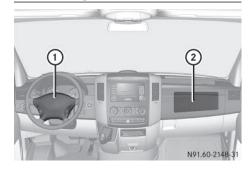
Driver's air bag (1) inflates in front of the steering wheel; co-driver's front air bag (2) inflates in front of and above the glove box and center console.
