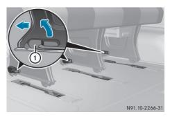
Locking mechanism lever on the feet of the bench
