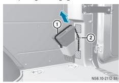
Wheel chock in the load/passenger compartment
