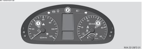
Instrument cluster in vehicles with steering-wheel buttons
