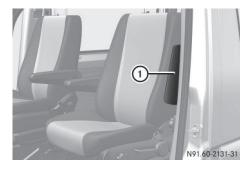
Thoraxbags ① are only installed for individual seats in the outer seat cushions of the driver's and co-driver's seats.
