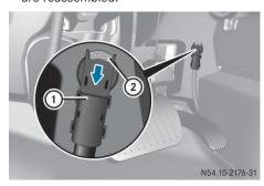
Battery isolating switch in the driver's footwell, on the right-hand side next to the accelerator pedal
