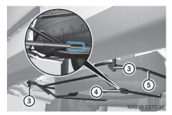
Spare wheel carrier under the vehicle
