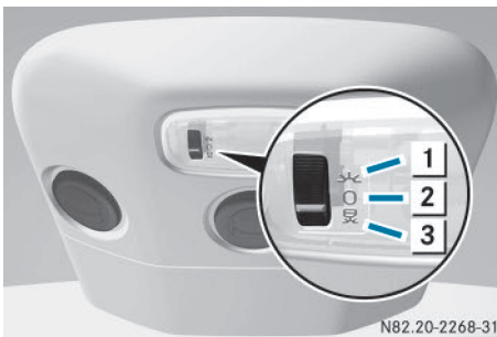
Interior light with switch (example: Passenger Van with rear-compartment air conditioning)
