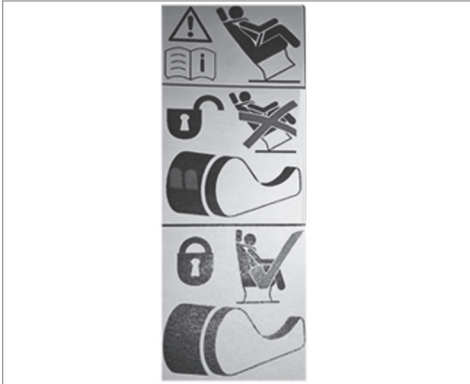
Warning on the rear bench seat with correctly installed rear bench seat shown.
